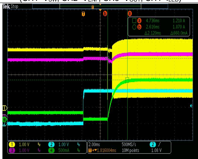
LED Current for Flash Off Waveform (CH1= V_{SW} , CH2= V_{ENF} , CH3= V_{OUT} , CH4= I_{LED} )
