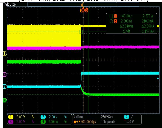
LED Current for Flash On Waveform (CH1= V_{SW} , CH2= V_{ENF} , CH3= V_{OUT} , CH4= I_{LED} )
