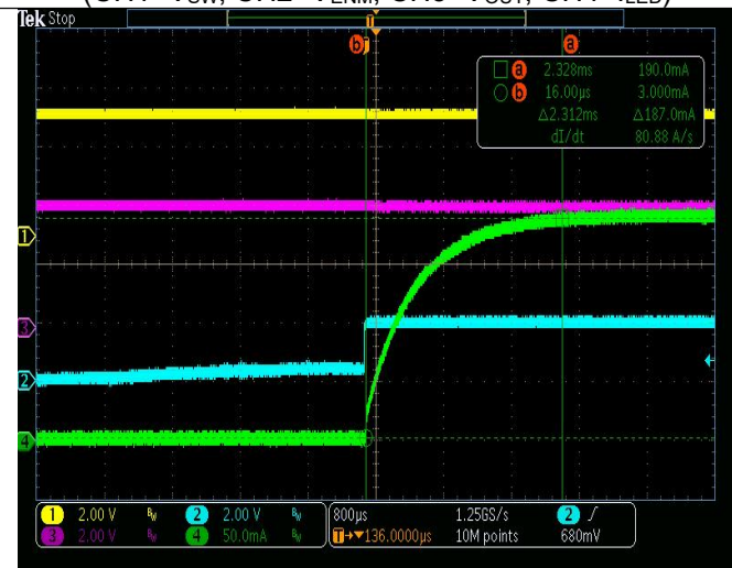
LED Current for Movie On Waveform (CH1= V_{SW} , CH2= V_{ENM} , CH3= V_{OUT} , CH4= I_{LED} )
