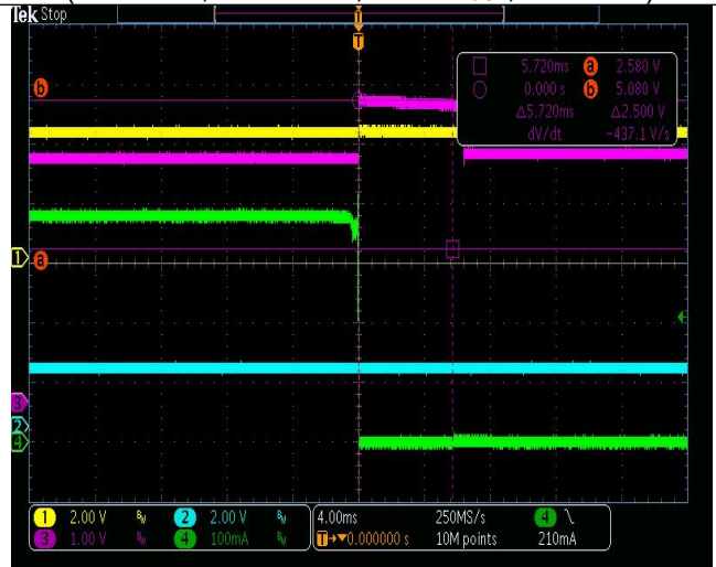
Open-LED Protection Waveform (CH1=V SW , CH2=V ENM , CH3=V OUT , CH4=I LED )
