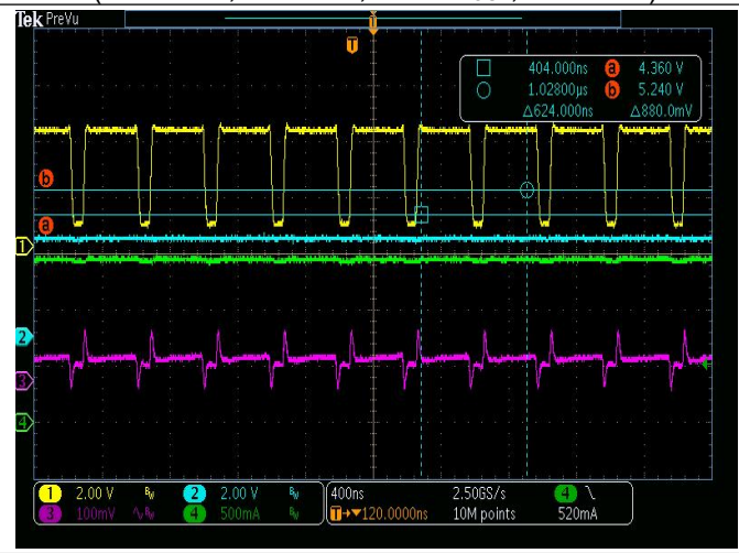
Flash Mode Switch Ripple Waveform (CH1= V_{SW} , CH2= V_{IN} , CH3= V_{OUT} , CH4= I_{LED} )
