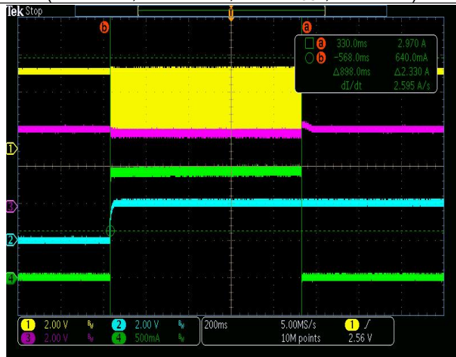
Flash Timeout Time Waveform (CH1=V SW , CH2=V ENM , CH3=V OUT , CH4=I LED )
