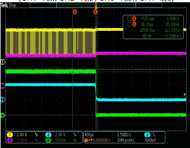
Short-LED Protection Waveform (CH1= V_{SW} , CH2= V_{OUT} , CH4= I_{LED1} )
